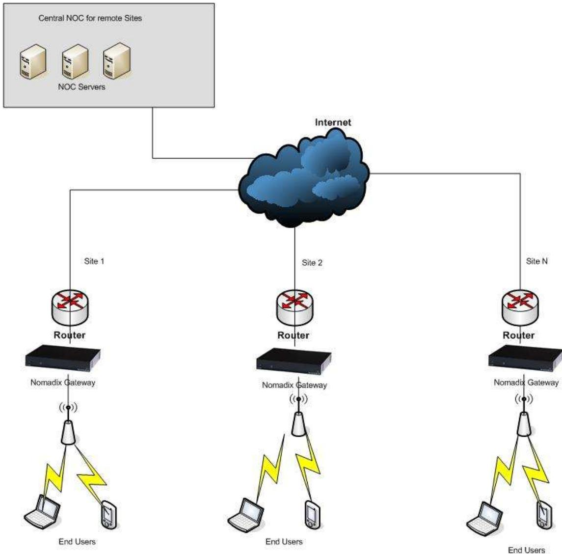
In this Scenario each hotspot consists of a simple Router, Nomadix Gateway and the Access Points required for the site. All of these devices can be managed and monitored from a central location based on the configurations needed. The HotSpots can also be linked together with the same Radius database. Either similar or different Portal Pages could be utilized for each HotSpot as well.
